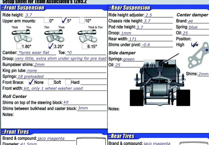
Diameter: 41.5mm Wheel: jaco Tire treatment: cs Treatment time: 15minutes Surface treated: just less than half Notes: clean tyre first with additive
